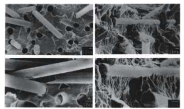
Figure 1: SEM Pictures of Glass Fiber Wetting & Coupling
